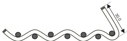
Plain wire hook ( for 8 & 10 mm thickness )
